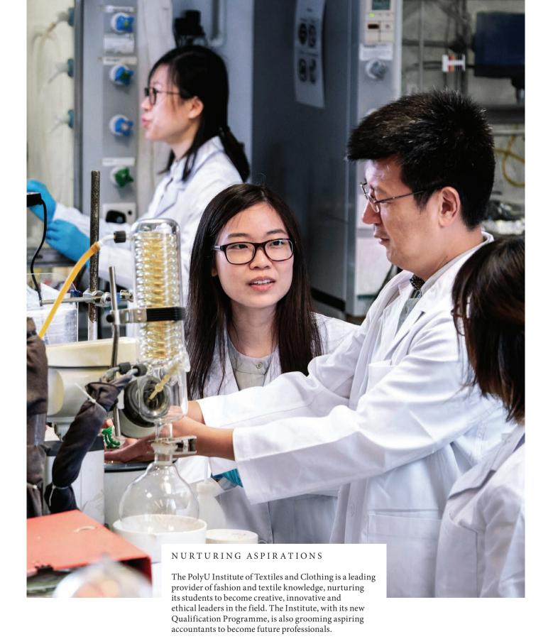
Pictured here is Associate Professor Bin Fei and his research students at the Material Synthesis and Processing Laboratory, where a rotary evaporator is used to purify flame retardants and smart dyes before being applied to various functional textiles.
